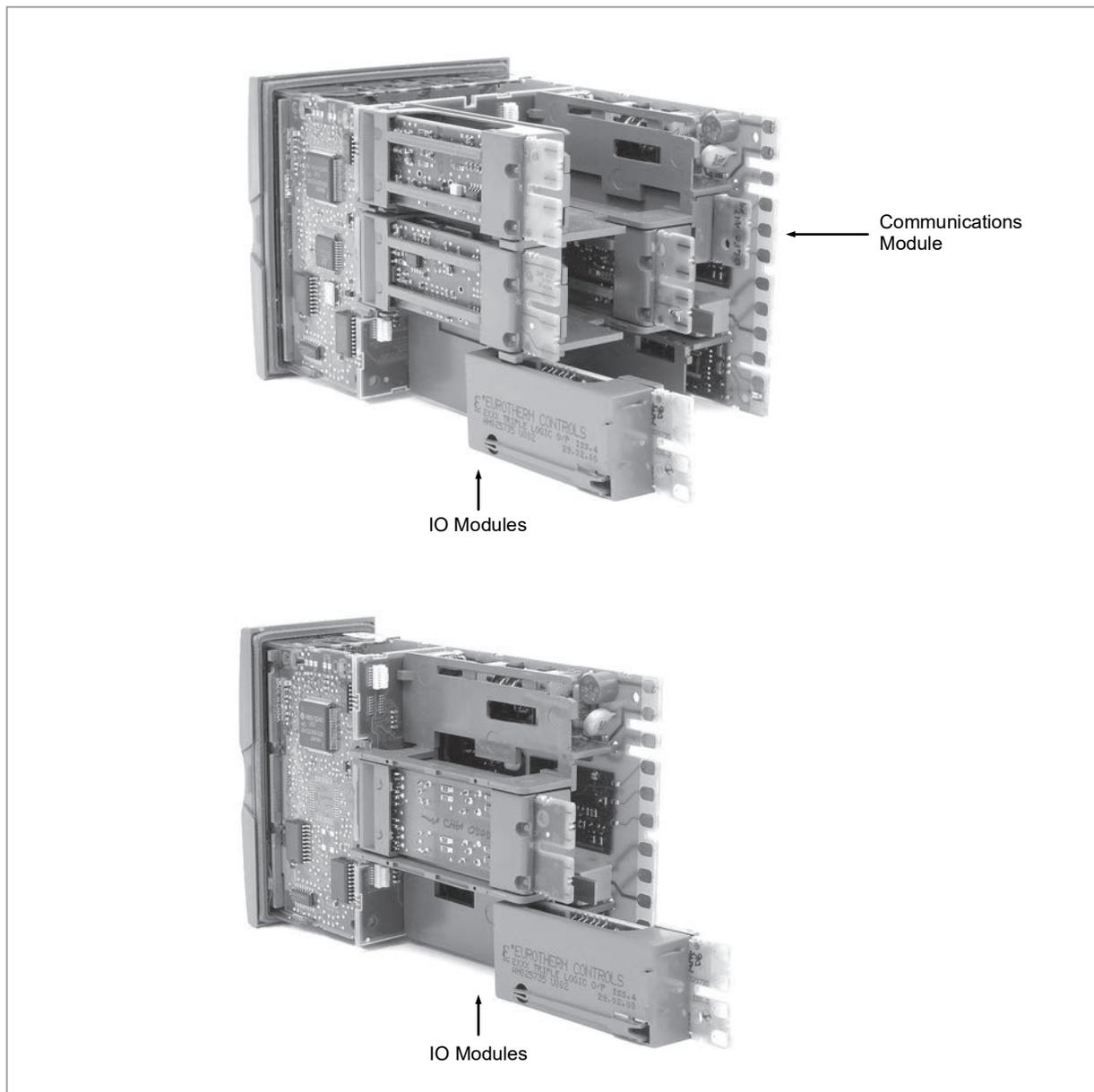
**Figure 34: View of the Plug-in Modules**
