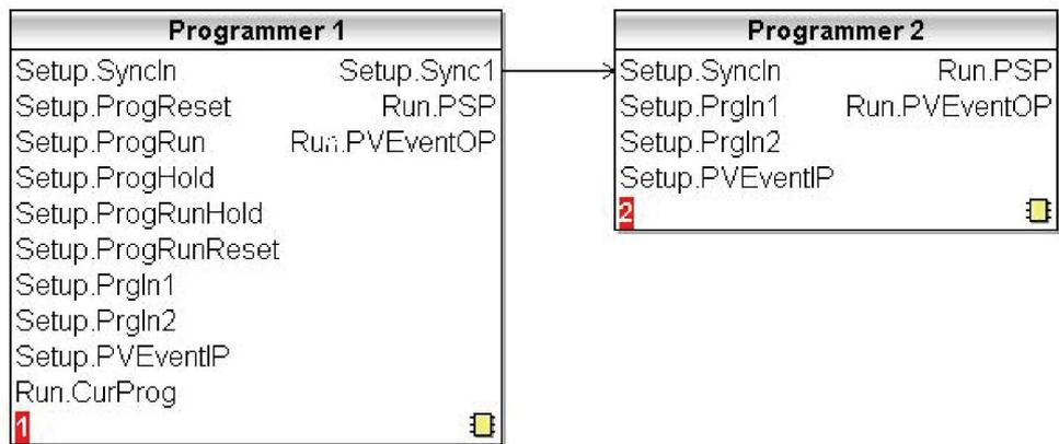
In this configuration, Programmer2 is a server to Programmer1. A program will have two profiles, Channel1 run by Programmer1 and Channel2 run by Programmer2. The program only needs to be loaded into the master programmer. To edit the program and to configure the programmers the following procedure should be followed:
