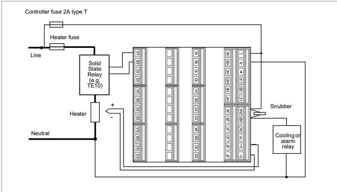
**Figure 14: Example Wiring Diagram**
