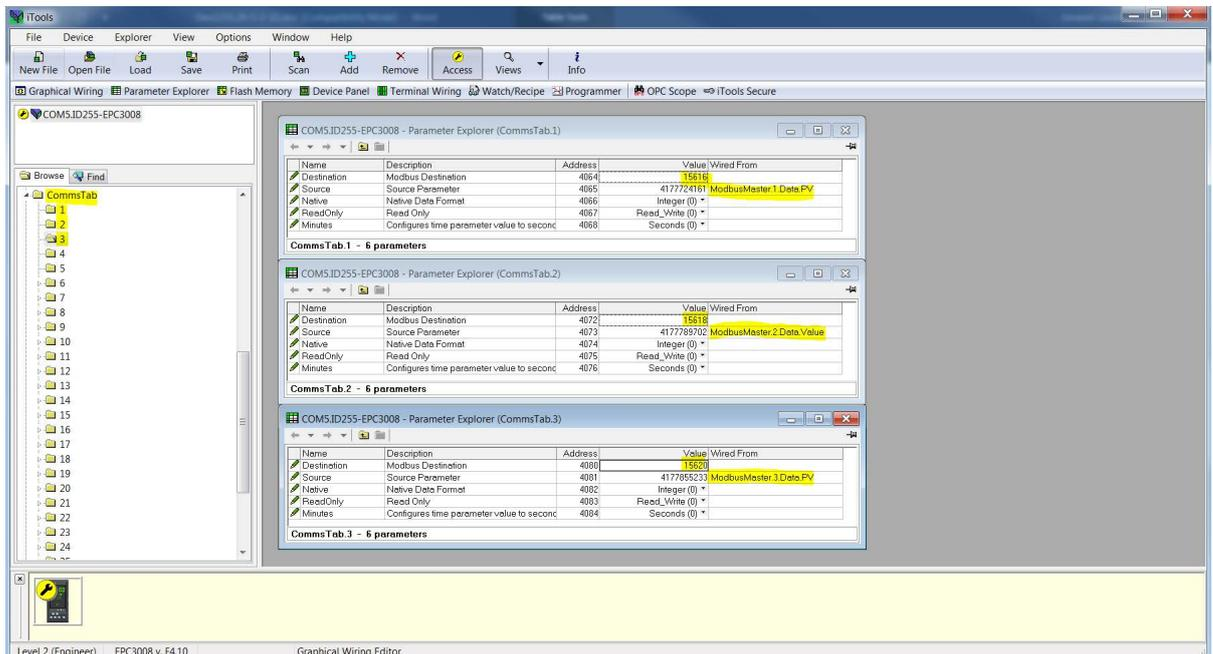
3. Screenshots below show MODBUS Client data auto-configured to appear at the MODBUS Indirection table and the values read by a 3rd party MODBUS Client from our MODBUS Client device:
