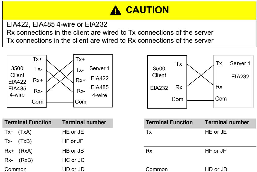
**Figure 41: Rx/Tx Connections for EIA422, EIA485 5-wire, EIA232**
