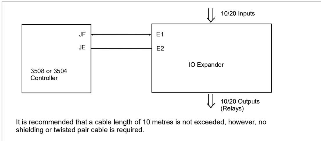
**Figure 37: IO Expander Data Transfer**
