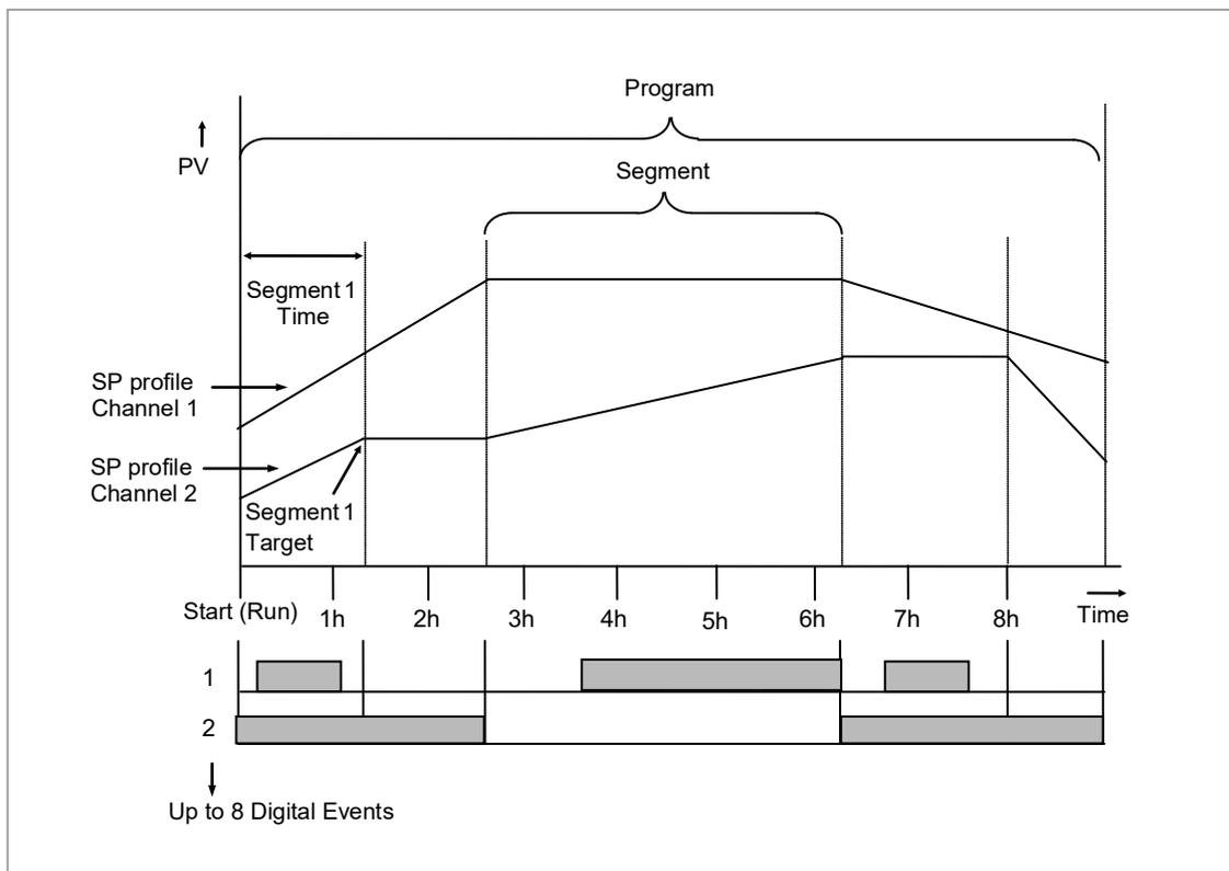
**Figure 74: Simple Two Profile Setpoint Program**
