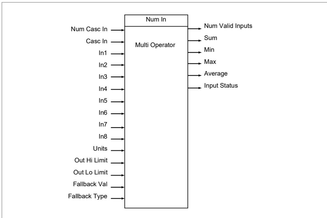
**Figure 55: Multi Input Operator Function Block**
