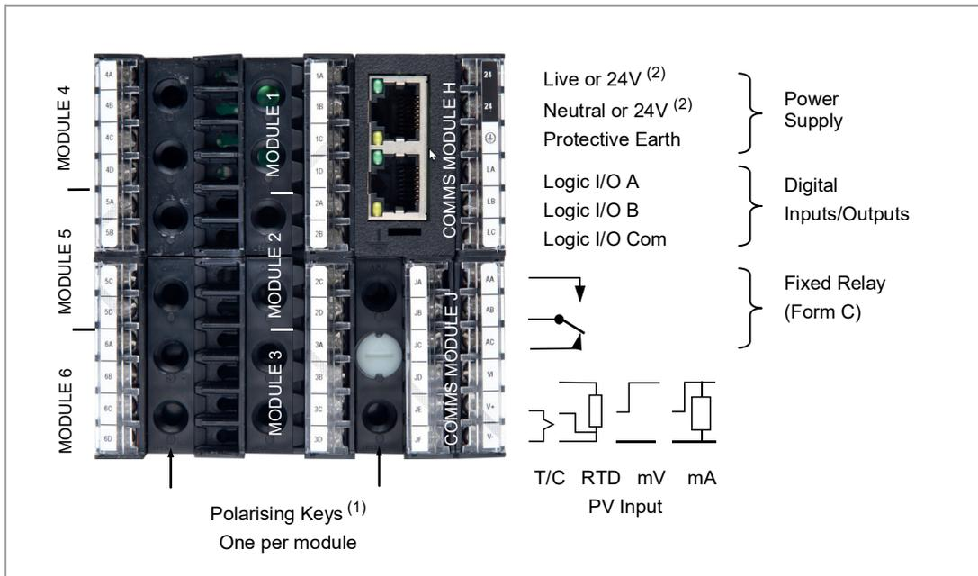
Figure 6: Rear Terminal View (with Serial or DeviceNet) – 3504 Controller
