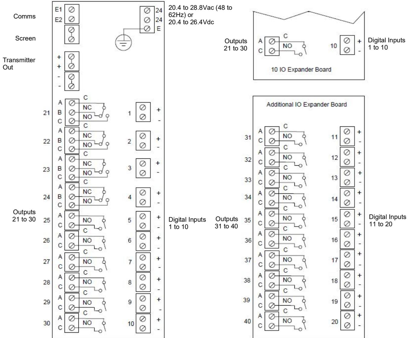
**Figure 13: IO Expander Terminals**
