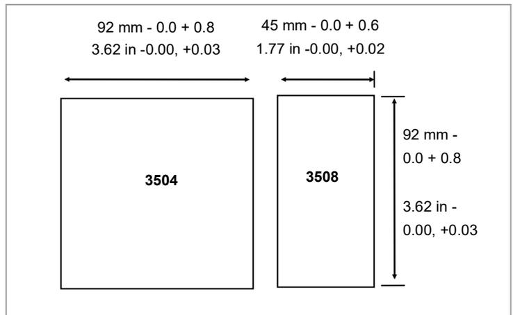
Figure 2: Panel Cut out Dimensions
