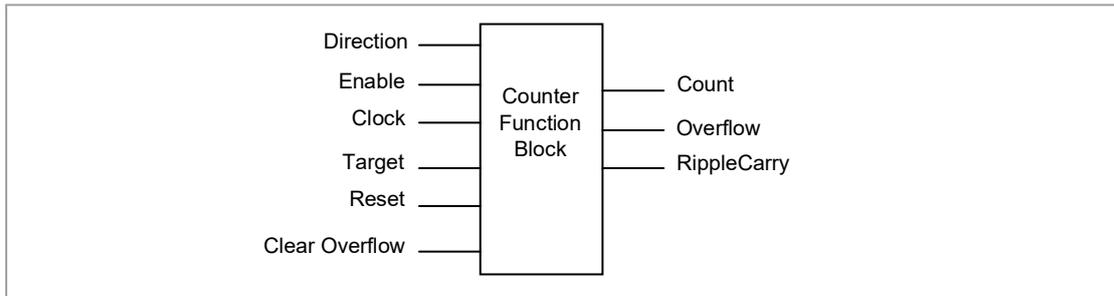
**Figure 43: Counter Function Block**
