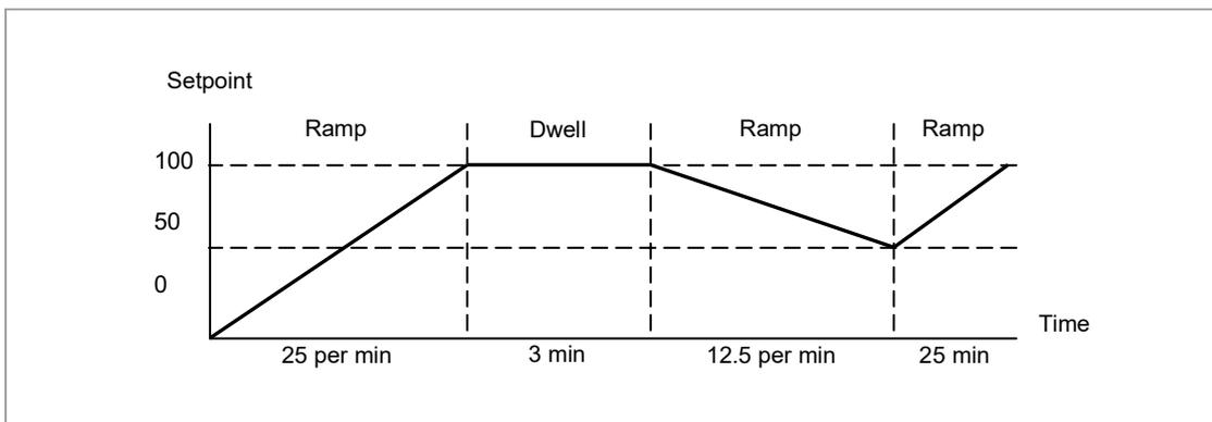
**Figure 76: Ramp Rate Programmer**
