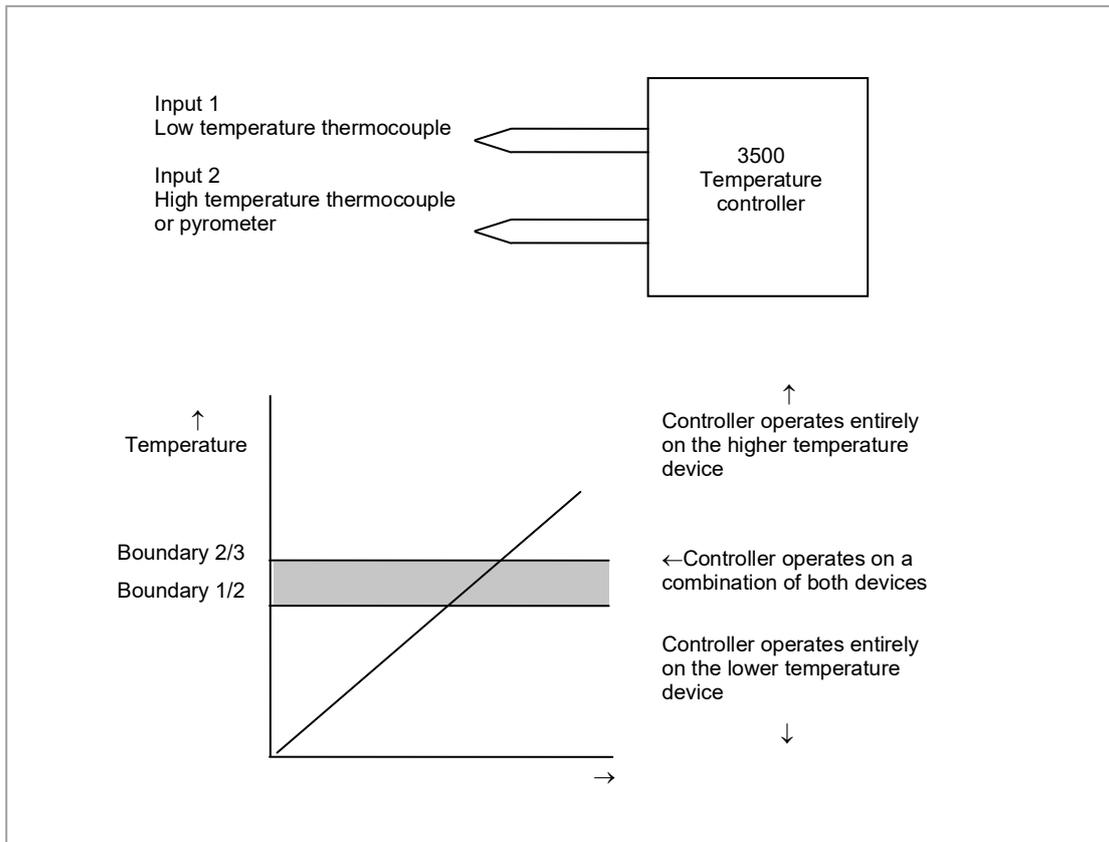
**Figure 78: Thermocouple to Pyrometer Switching**
