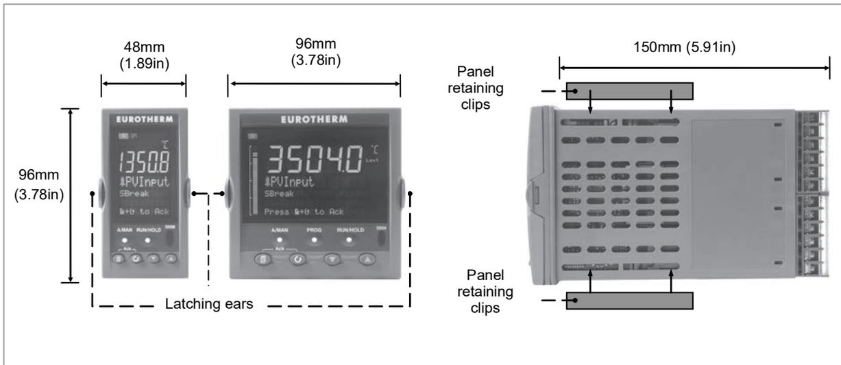
Figure 1: Controller Dimensions
