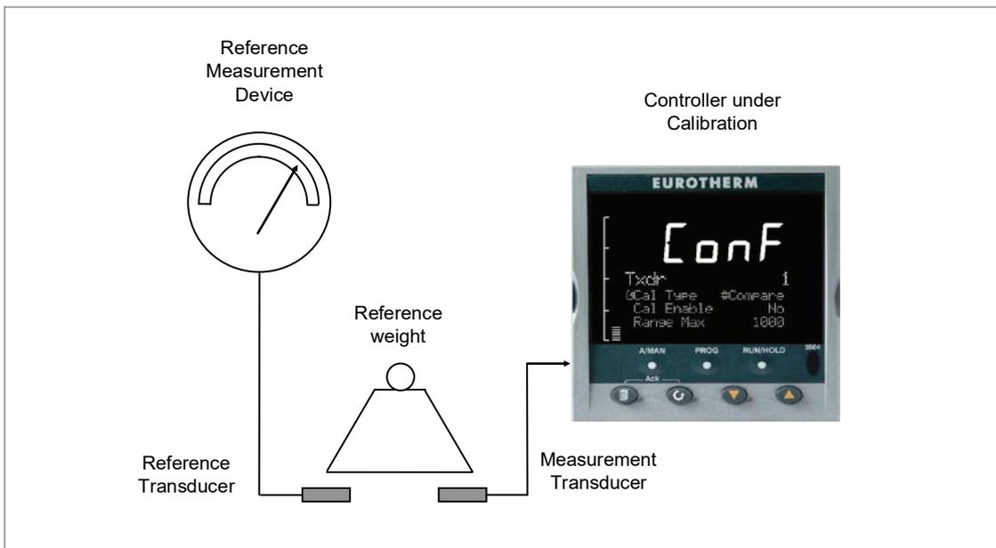
**Figure 84: Comparison Calibration**
