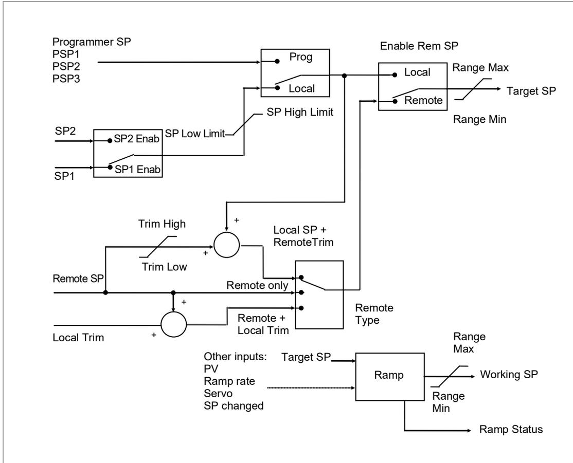
Figure 68: Setpoint Function Block
