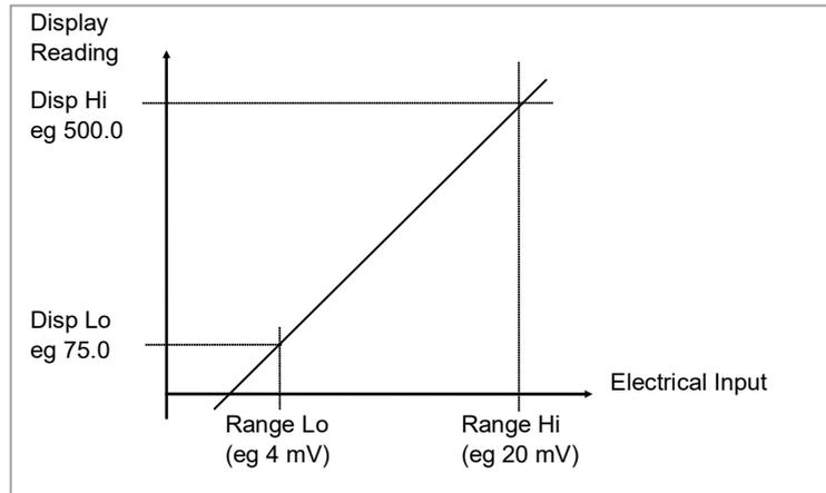
Figure 30: PV Input Scaling
