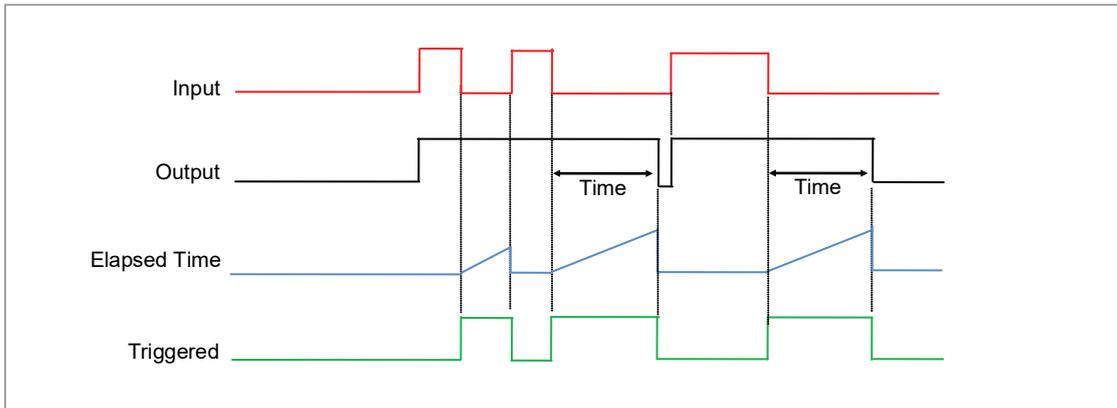
**Figure 49: Minimum On Timer Under Different Input Conditions**
