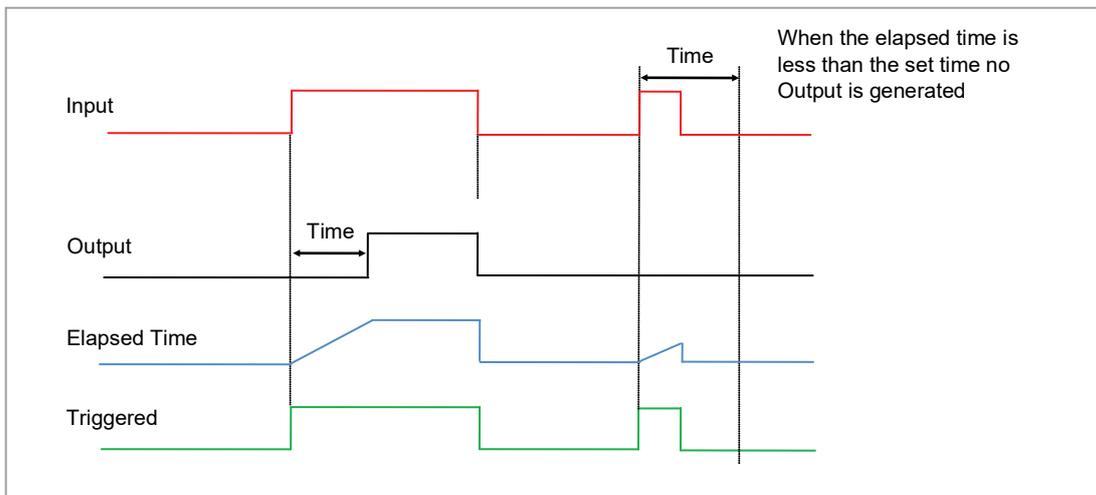
**Figure 47: On Delay Timer Under Different Input Conditions**
