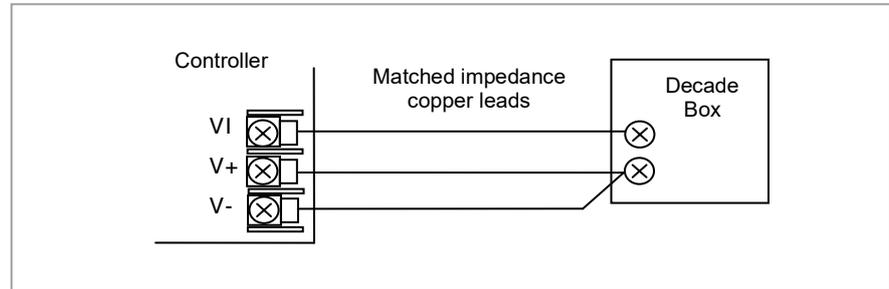
**Figure 87: Connections for RTD Calibration**
