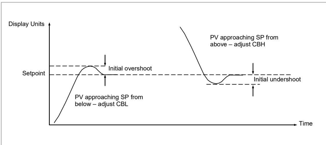
Figure 67: Manual Setting of Cutback
