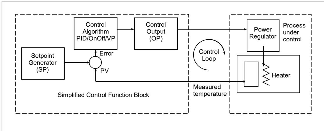
**Figure 57: Single Loop Single Channel**
