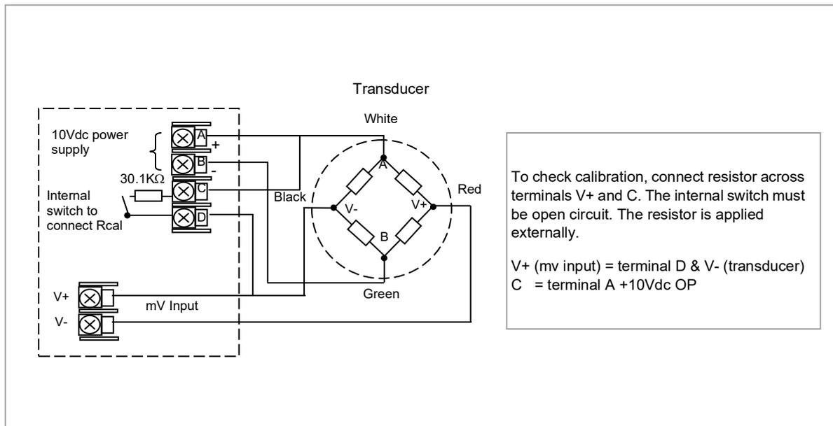
**Figure 81: Strain Gauge Wiring Diagram - Internal Calibration Resistor**
