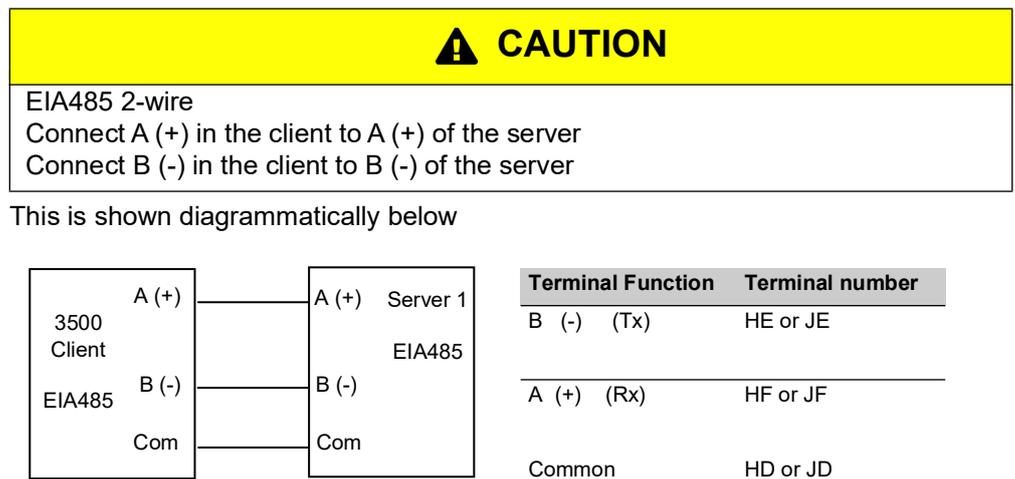
**Figure 42: : Rx/Tx Connections EIA485 3-wire**
