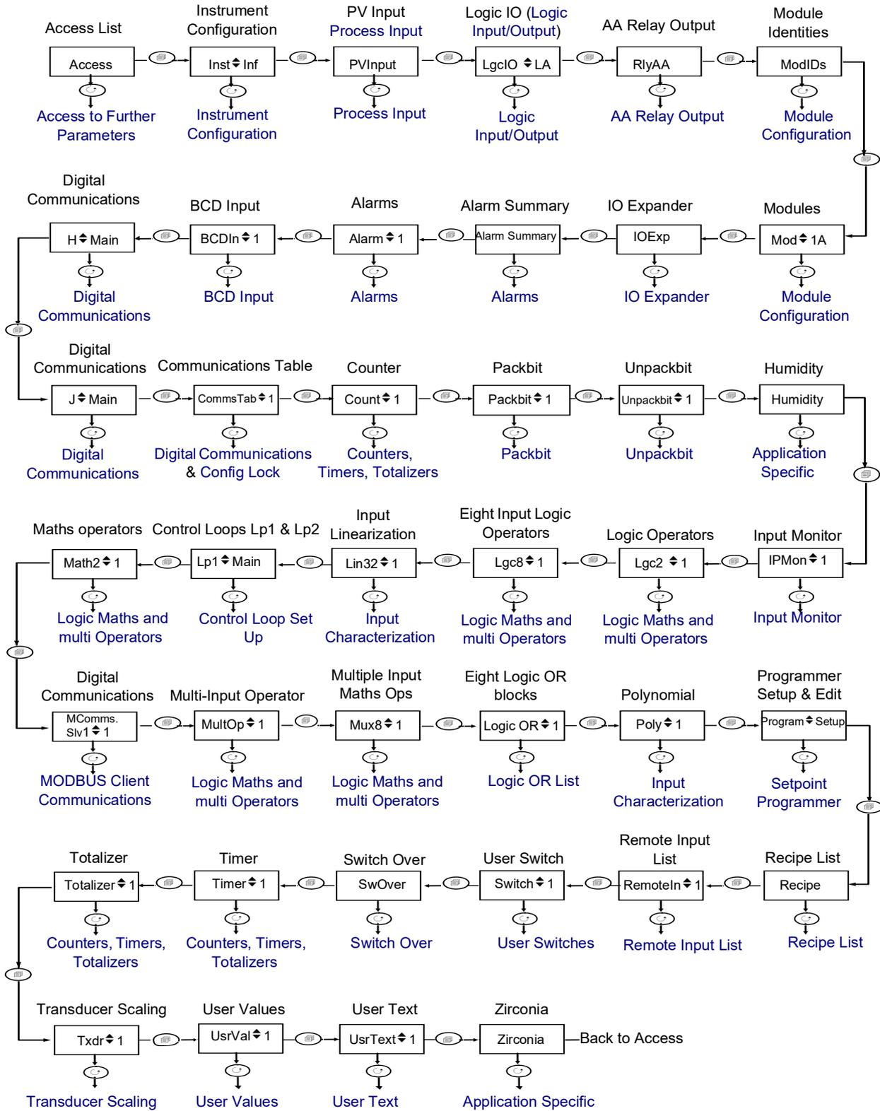
Figure 25: Navigation Diagram
