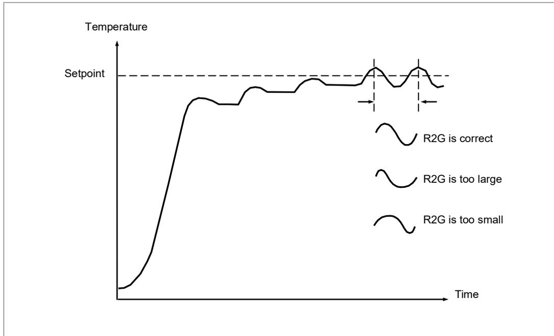
Figure 66: Setting Relative Cool Gain
