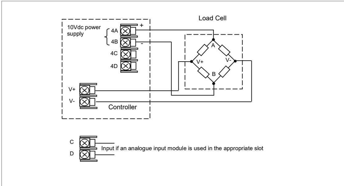
Figure 83: Load Cell Wiring Diagram
