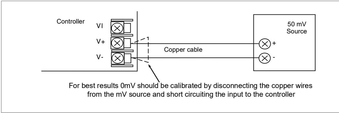
**Figure 88: Connections for mV Calibration**
