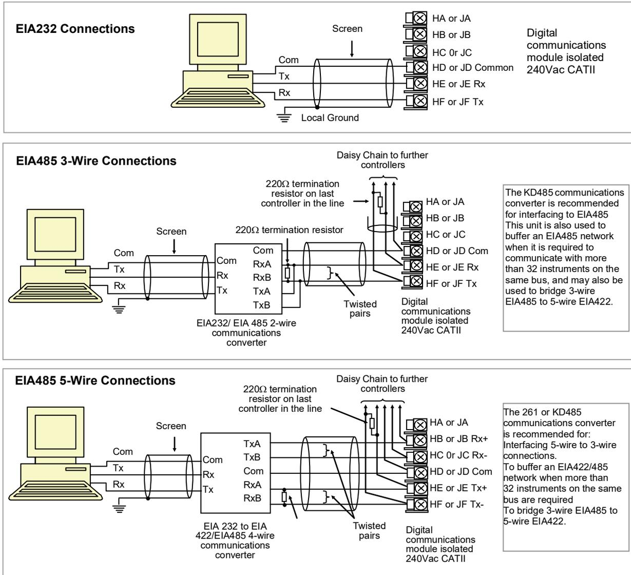
Figure 10: EIA232 and EIA485 Connections
