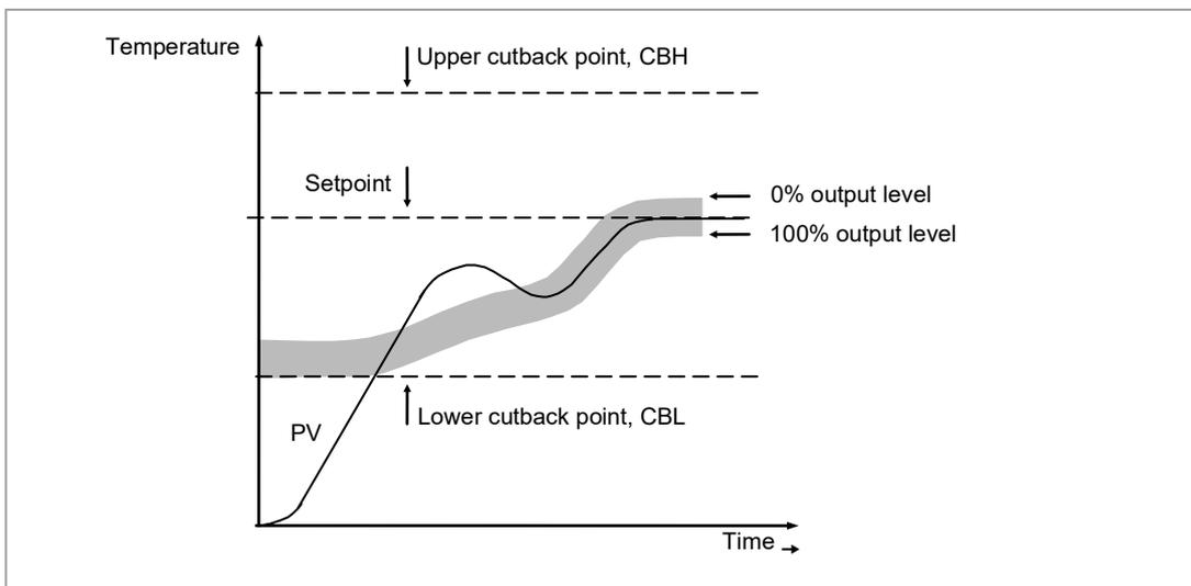
Figure 61: High and Low Cutback
