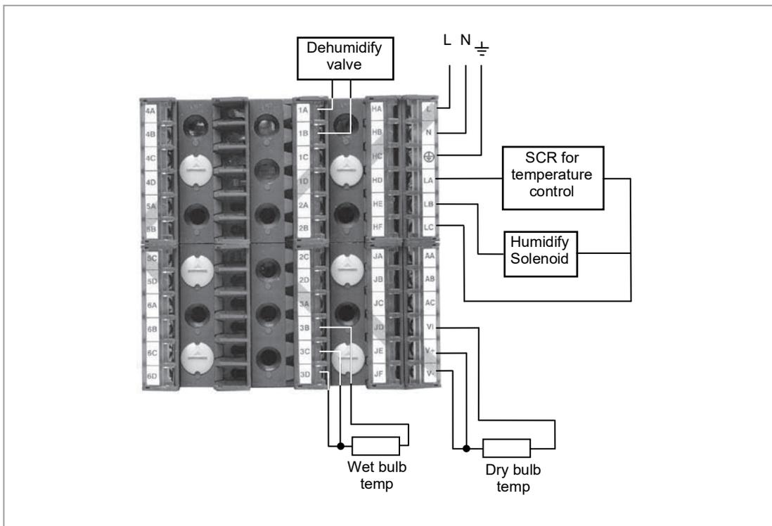
**Figure 50: Example of Humidity Controller Connections**
