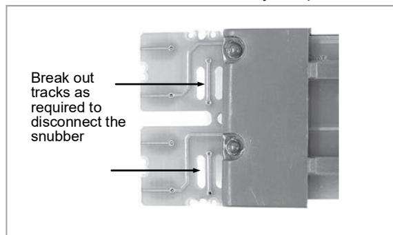
**Figure 15: Snubber Removal**
