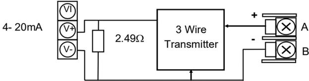
Isolated Transmitter Option module +24Vdc >20mA
