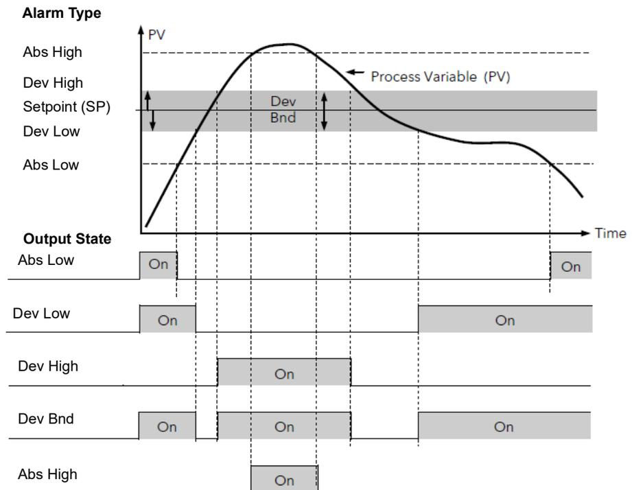
Figure 38 Analog Alarm Types
