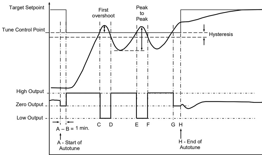
Figure 63: Autotune - Heat/Cool Process
