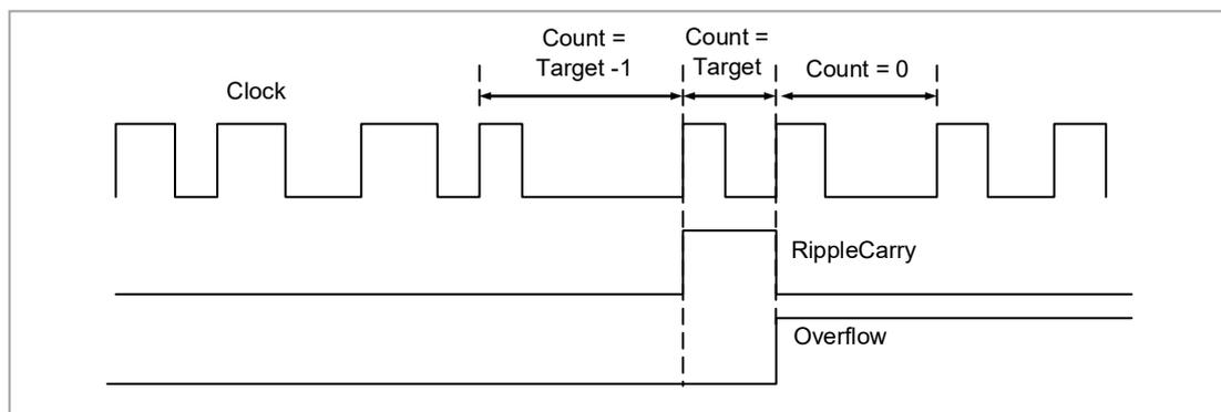
Figure 45: : Timing Diagram for an Up Counter
