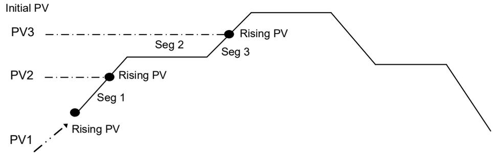
The user may specify the start point based on a Rising PV as shown in the diagram above or on a Falling PV as shown below depending on type of profile being run.
