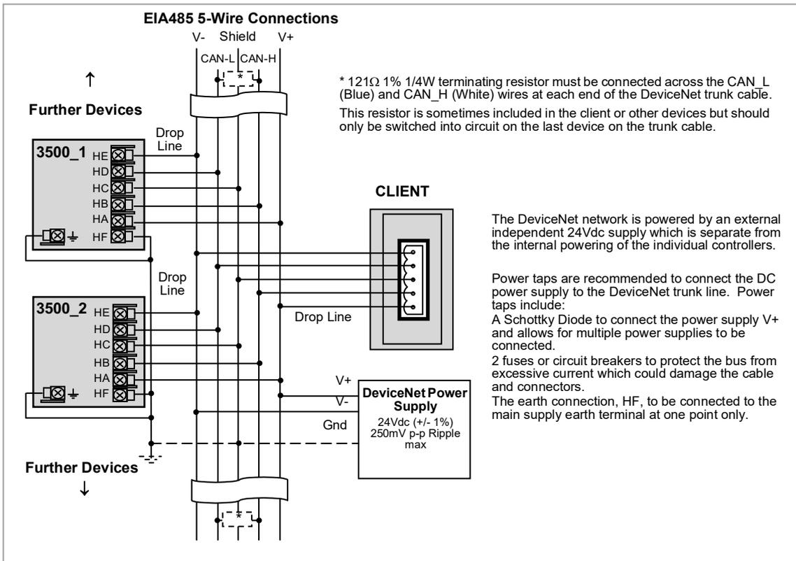
Figure 11: Example of DeviceNet Wiring
