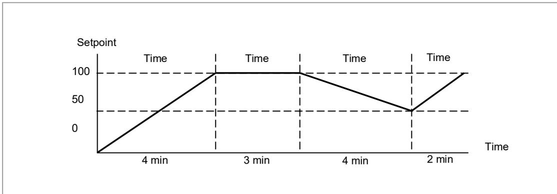
**Figure 75: All Segments Configured as Time-to-Target**
