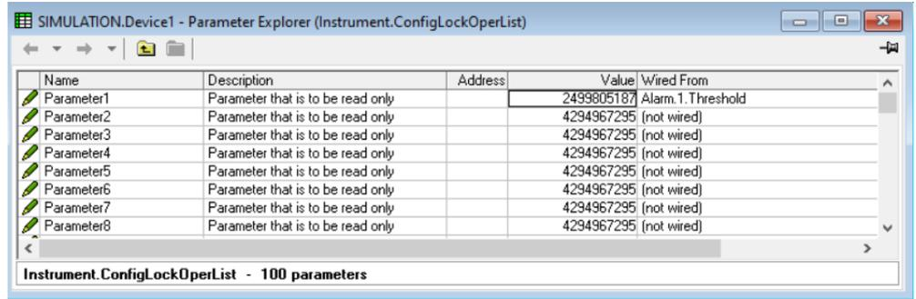
The example shows the first 8 of 100 parameters of which the first has been selected as 'Alarm 1 Threshold'. This parameter is to be read only when Config Lock is enabled and the controller is in Operator access level.
