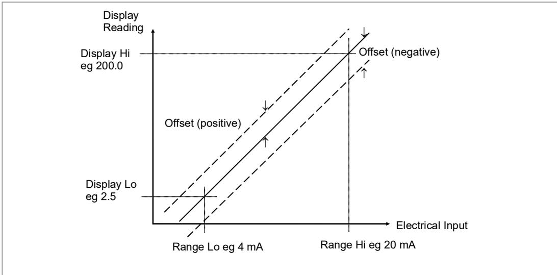
**Figure 35: Input Scaling (Standard IO)**
