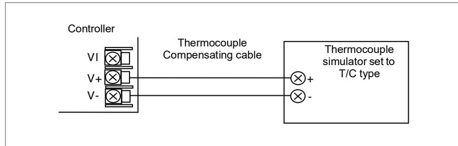
**Figure 86: Connections for Thermocouple Calibration**
