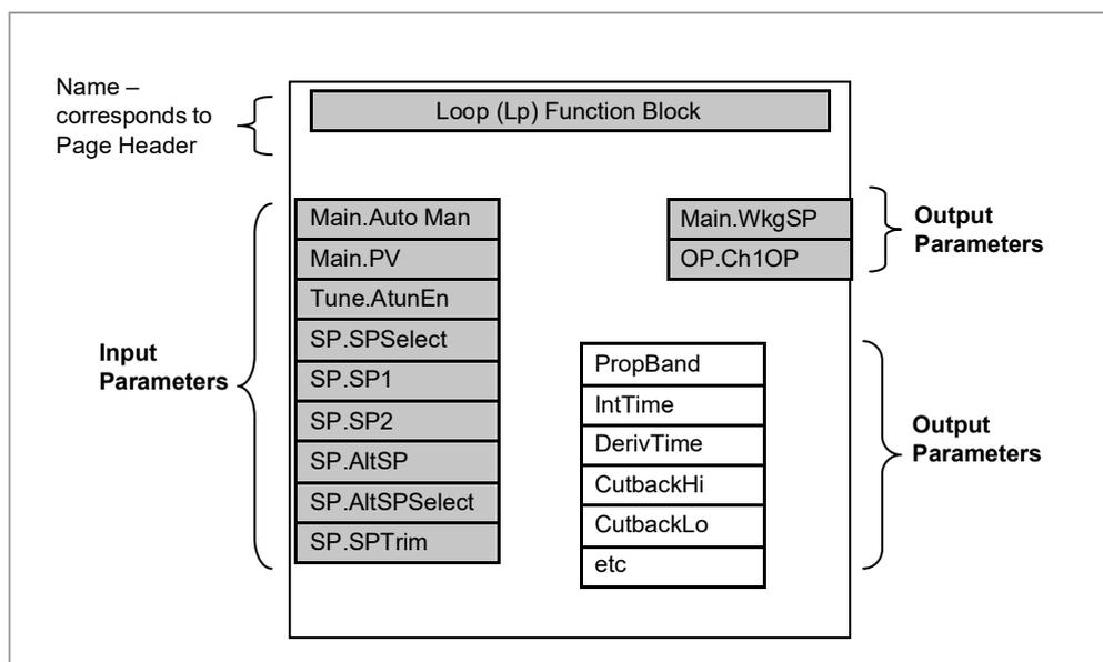
**Figure 21: Example of a Function Block**
