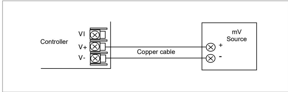
**Figure 85: Connections for mV Calibration**
