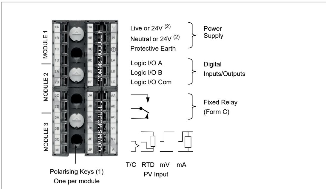
Figure 4: Rear Terminal View (with Serial or DeviceNet) – 3508 Controller
