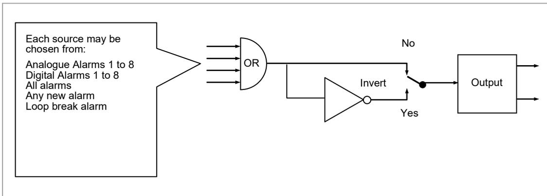
Figure 39 Attaching an Alarm to Operate an Output
