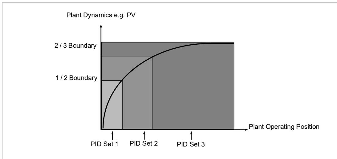
**Figure 62: Gain Scheduling over a Wide range of Operating Variable**
