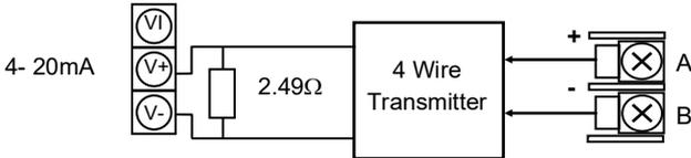
Isolated Transmitter Option module +24Vdc >20mA
