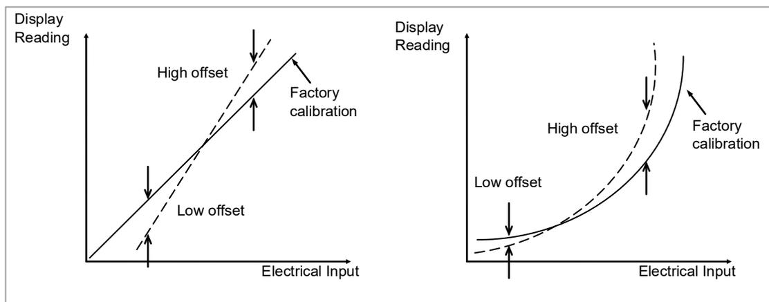
Figure 32: Two Point Offsets
