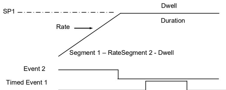
1. In 'Program Setup' select the channel to be set up using ⏴ or ⏵. For convenience it is also possible to toggle between Ch1 and Ch2 using the
