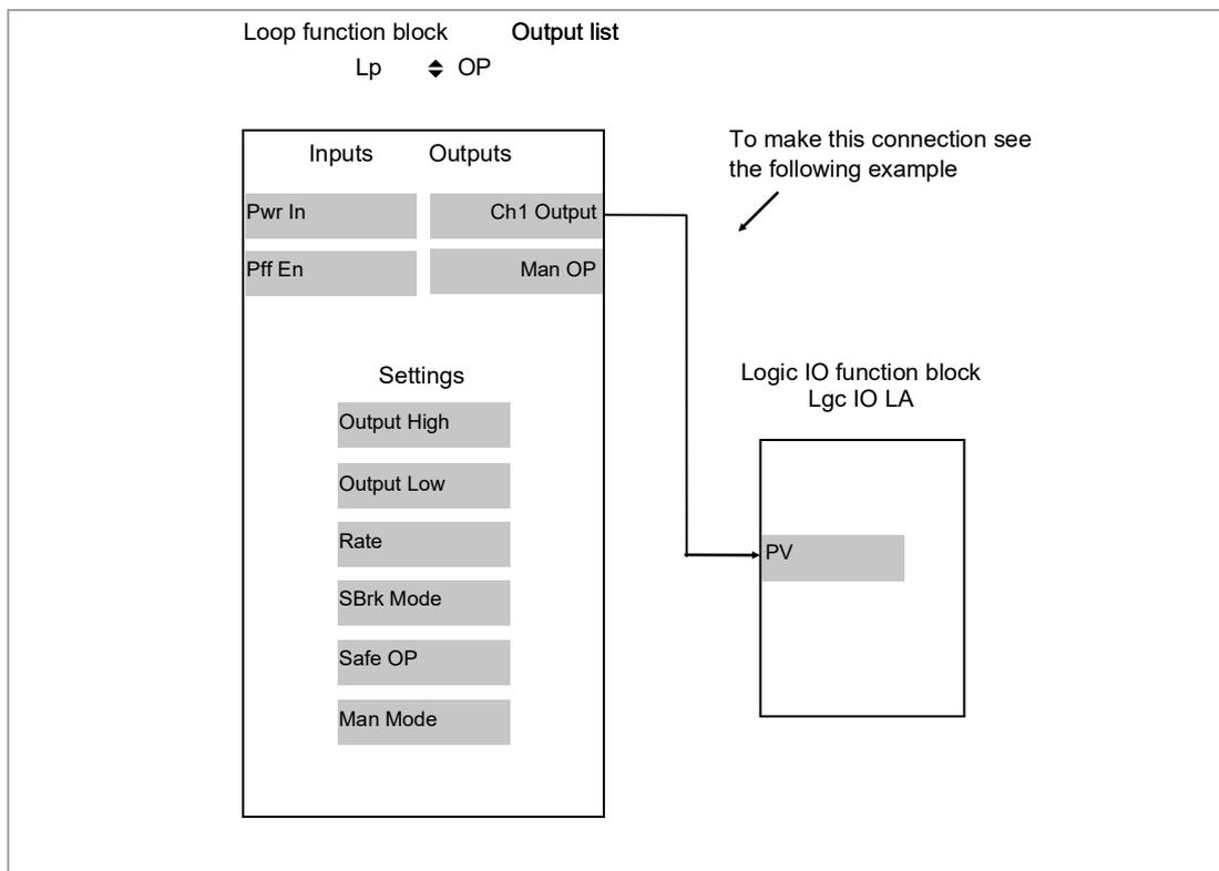
Figure 27: Function Block Wiring
