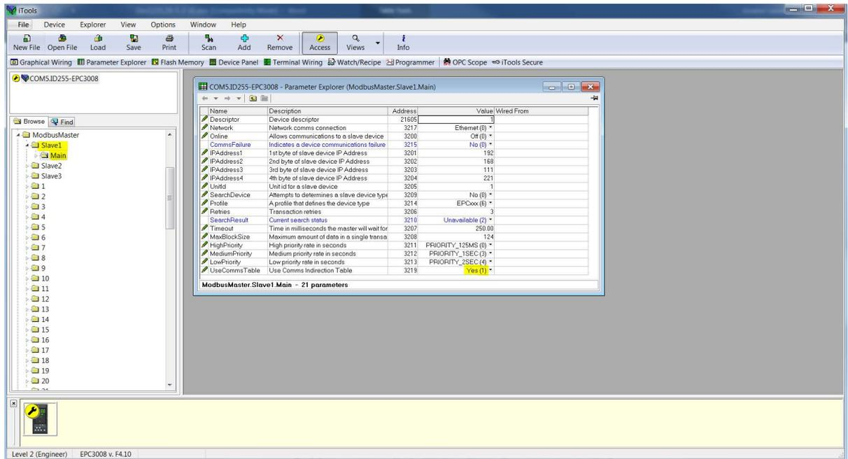
2. In Operator mode, the CommsTab Function Block should now show every configured MODBUS Client data. The user can then change Native, ReadOnly and Minutes parameters from default to configure how the data is presented from the MODBUS indirection table.
