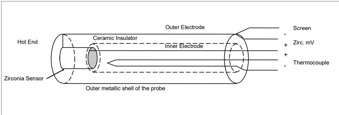
Figure 8: Zirconia Probe Wiring
