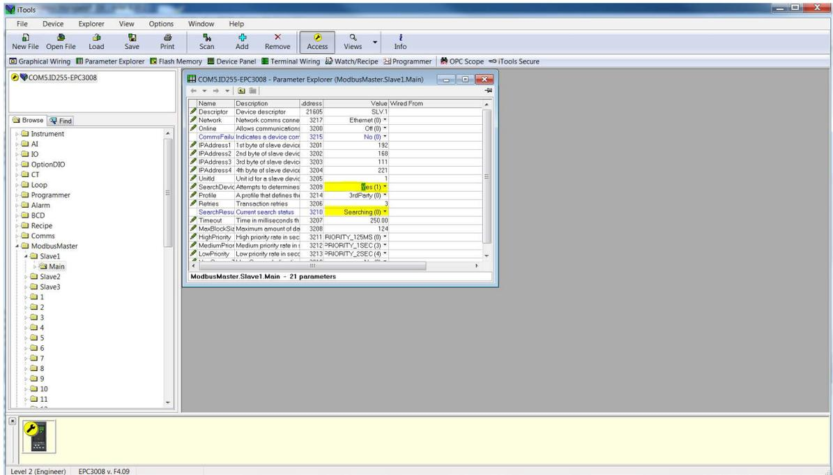
4. If the MODBUS server is online then the search result will be “Available(1)” otherwise the result will be “Unreachable(3)”. If it is a Eurotherm instrument with a supported profile, the “Profile” parameter will display the MODBUS server’s profile otherwise it will display “3rdParty(0)”.
