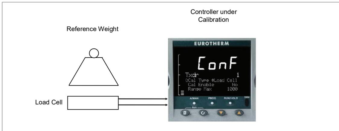
Figure 82: Load Cell
