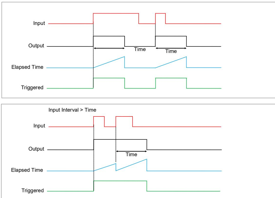
**Figure 46: On Pulse Timer Under Different Input Conditions**
