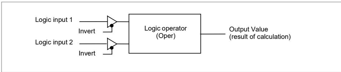
**Figure 51: 2 Input Logic Operators**
