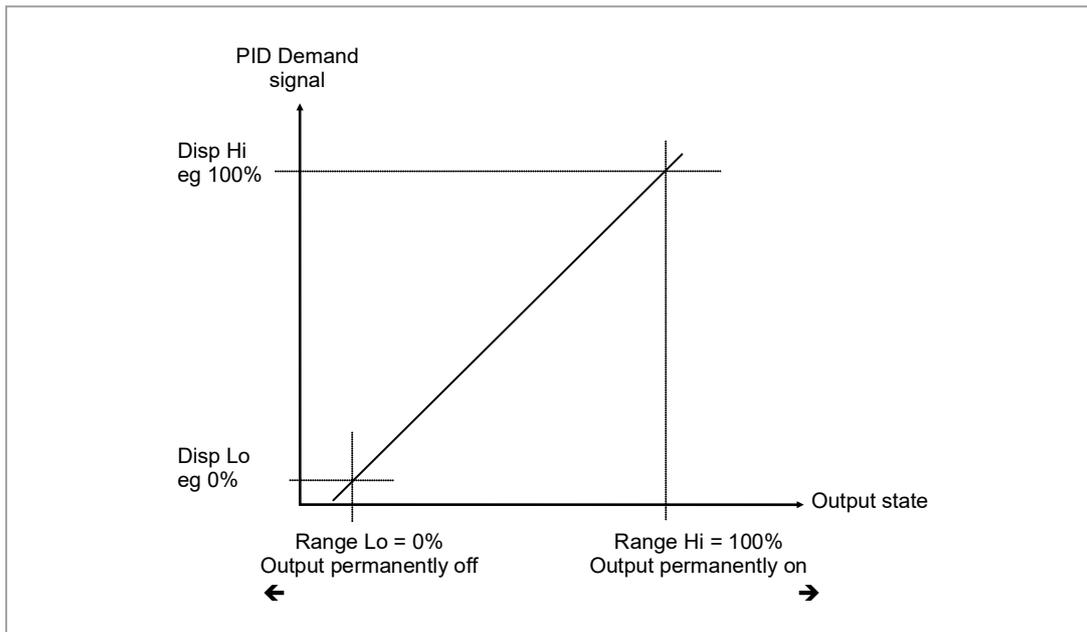
**Figure 36: Time Proportioning Output**
