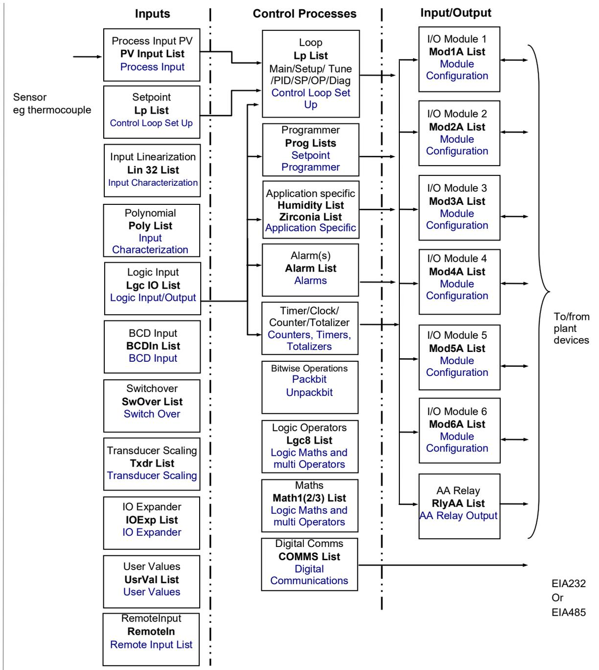
Figure 26: Controller Example
