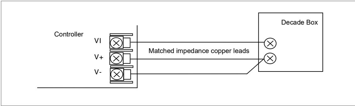
Figure 90: Connections for RTD Calibration
