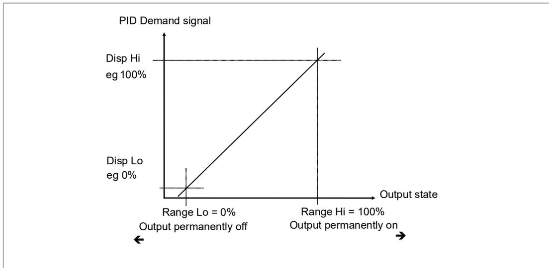
Figure 33: Scaling a Logic Output
