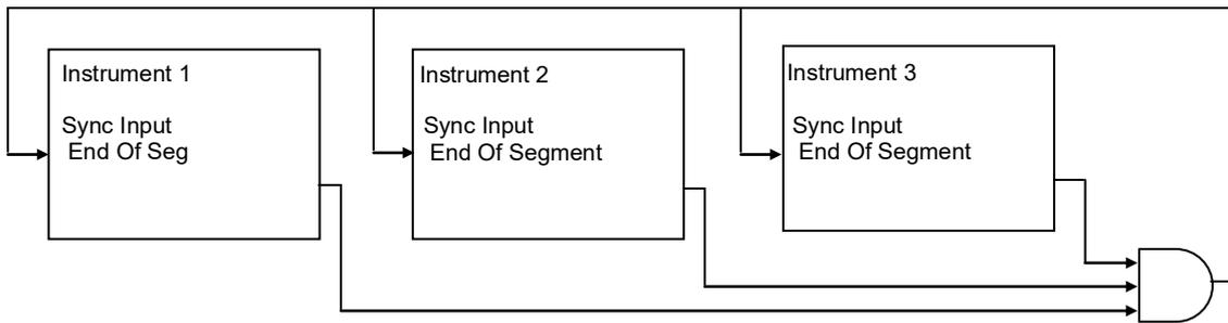
At the end of a segment, the program will be put into a temporary hold state (program status will continue to show that the program is running), the hold beacon will flash, the end\_of\_segment parameter will be true. Once all segments have completed, the SyncInput goes high and the next segment is started.
