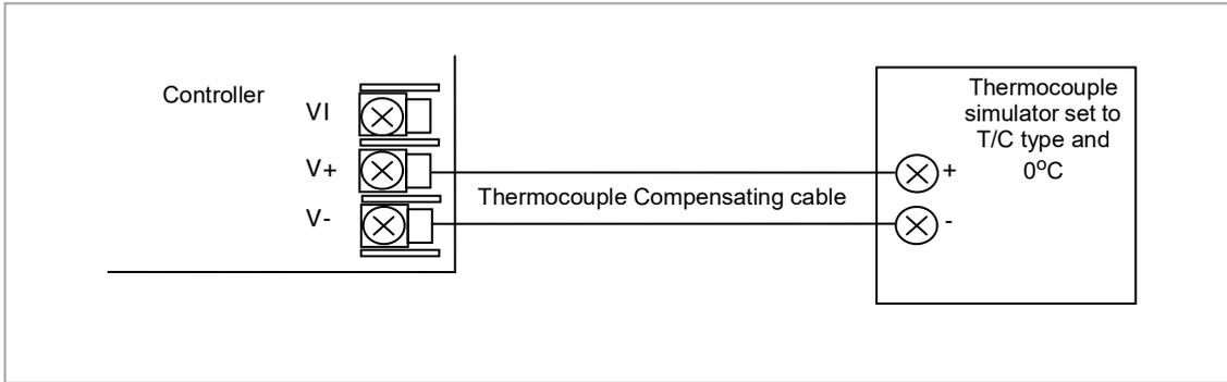
**Figure 89: Connections for Thermocouple Calibration**
