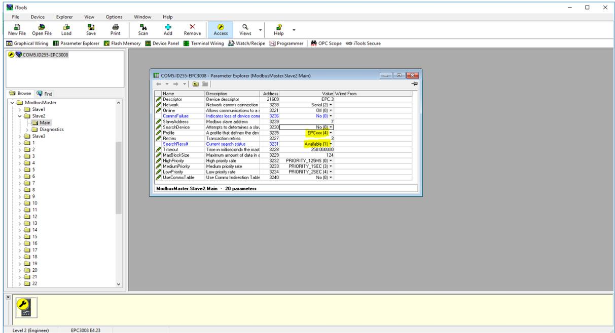
8. For the third server (ModbusMaster>Slave3>Main), we can configure a serial server with an unsupported profile by configuring the MODBUS server address and then starting “SearchDevice”.
