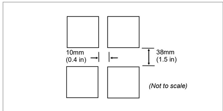
**Figure 3: Minimum Spacing Between Controllers**
