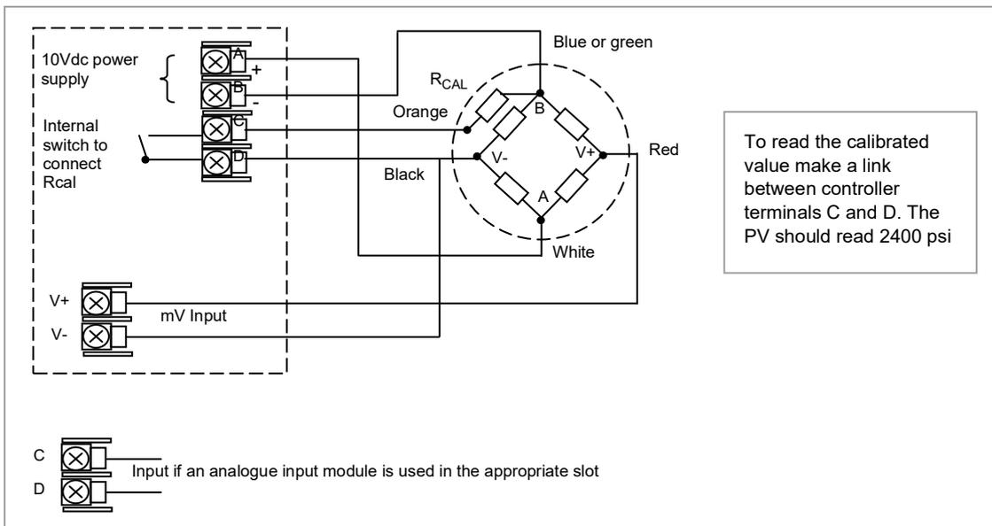
**Figure 80: Pressure Transducer Wiring Diagram**
