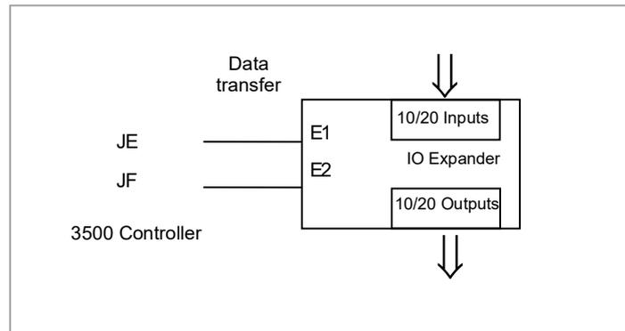
**Figure 12: Data Transfer Between IO Expander and Controller**
