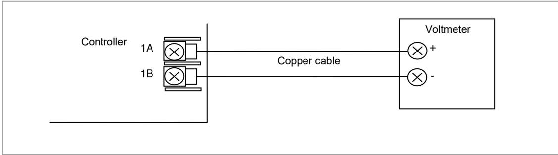
**Figure 91: Calibration of DC Output Module**
