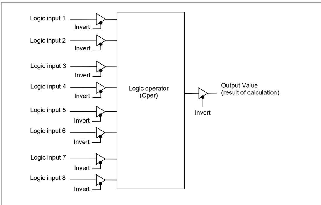
**Figure 52: 8 Input Logic Operators**
