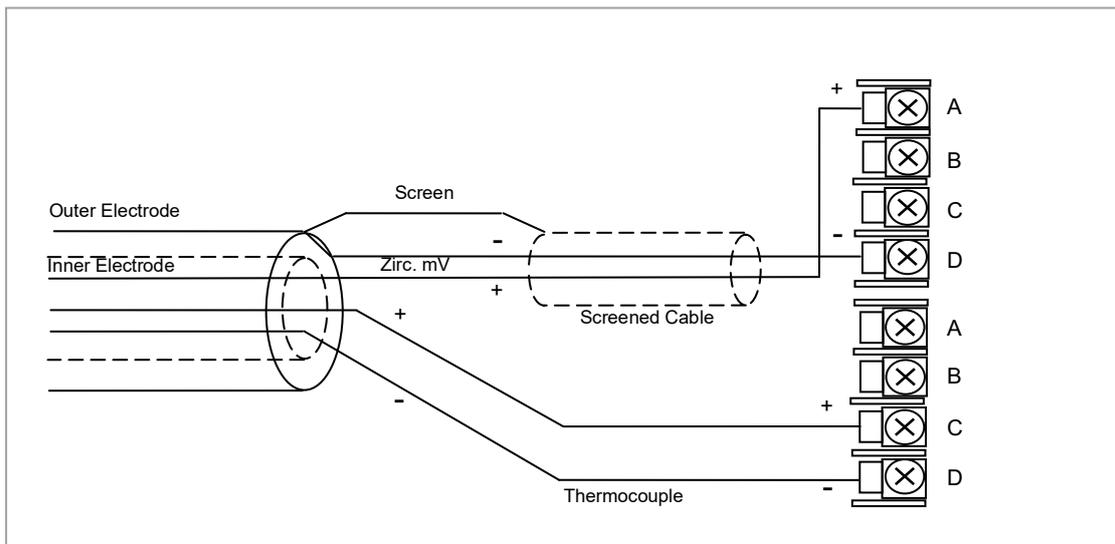
Figure 9: Zirconia Probe Wiring
